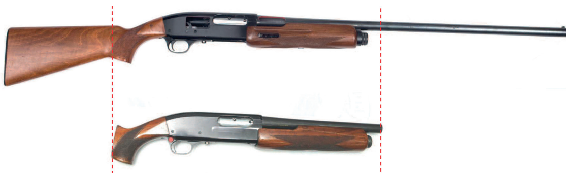
Fig. 6-1. Comparison between a full-size pump-action shotgun (top) and the one Monis carried; dotted lines indicate cuts
